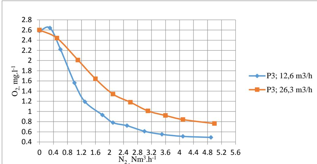
FIG.7. Comparison of oxygen concentration at different flow rates of wine in the visor P3.
