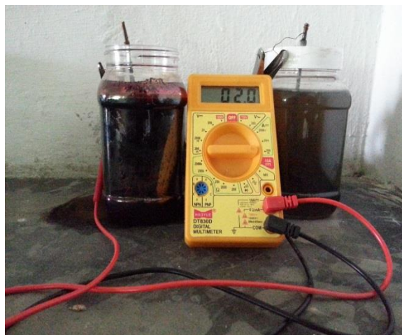
FIG. 2. Photographic picture of the experimental MFC set up.
