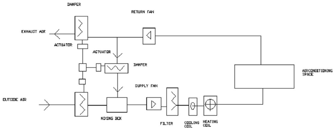
**Fig. 4: Schematic representation of single zone VAV system**
