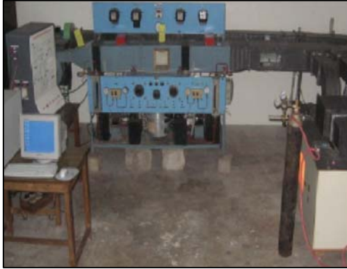
Fig. 6: Photographic view of VAV Air system conditioning
