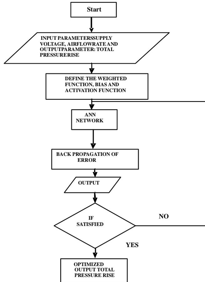
**Fig. 3: Flow chart for neuron model of fan**
