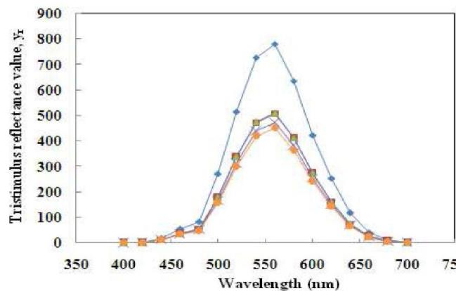
**Figure 2 :** Variation of the tristimulus reflectance value ( $y_r$ ) with wavelength for PMMA/AREAPP composites. (◆) 100/0, (■) 98/2, (▲) 96/4, (✗) 94/6 and (●) 92/8 (wt/wt%)
