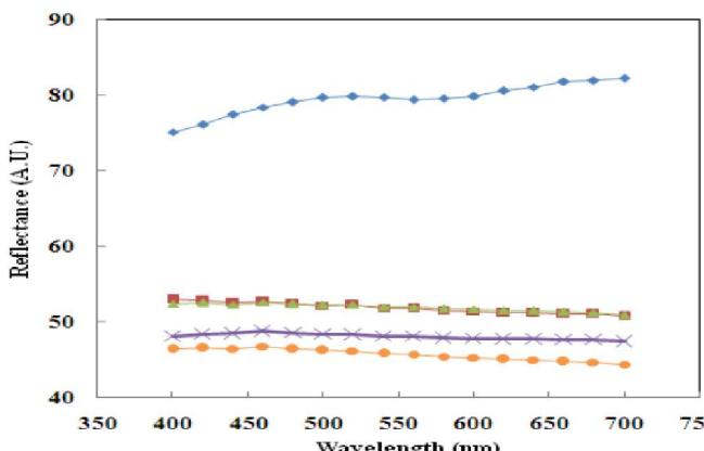
**Figure 1 :** The change in reflection percentage (R%) spectra for PMMA/AREAPP composites. (◆) 100/0, (■) 98/2, (▲) 96/4, (✗) 94/6 and (●) 92/8 (wt/wt%)
