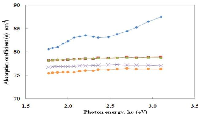
**Figure 6 :** The absorption coefficient ( $\alpha$ ) of PMMA/AREAPP composites as a function of photon energy ( $h\nu$ ). (◆) 100/0, (■) 98/2, (▲) 96/4, (✗) 94/6 and (●) 92/8 (wt/wt%)
