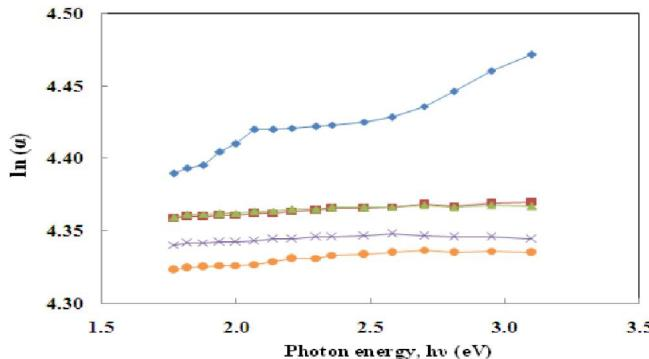
**Figure 7 :** Urbach law plots for PMMA/AREAPP composites. (◆) 100/0, (■) 98/2, (▲) 96/4, (✗) 94/6 and (●) 92/8 (wt/wt%)
