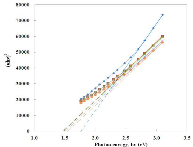
**Figure 8 :** The variation of  $(\alpha h\nu)^2$  for PMMA/AREAPP composites as a function of photon energy ( $h\nu$ ). (◆) 100/0, (■) 98/2, (▲) 96/4, (✗) 94/6 and (●) 92/8 (wt/wt%)
