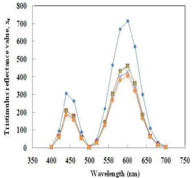
**Figure 3 :** Variation of the tristimulus reflectance value ( $x_r$ ) with wavelength for PMMA/AREAPP composites. (◆) 100/0, (■) 98/2, (▲) 96/4, (✗) 94/6 and (●) 92/8 (wt/wt%)
