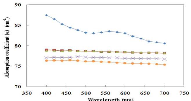
**Figure 5 : The absorption coefficient ( $\alpha$ ) of PMMA/AREAPP composites as a function of wavelength. (◆) 100/0, (■) 98/2, (▲) 96/4, (×) 94/6 and (●) 92/8 (wt/wt%)**
