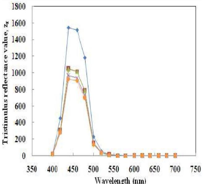
**Figure 4 :** Variation of the tristimulus reflectance value ( $z_r$ ) with wavelength for PMMA/AREAPP composites. (◆) 100/0, (■) 98/2, (▲) 96/4, (✗) 94/6 and (●) 92/8 (wt/wt%)
