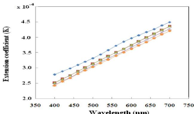
**Figure 10 : Variation in the extinction coefficient (K) as a function of wavelength ( $\lambda$ ) for PMMA/AREAPP composites. (◆) 100/0, (■) 98/2, (▲) 96/4, (×) 94/6 and (●) 92/8 (wt/wt%)**
