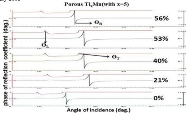
FIG. 2. Experimental phase of the reflection coefficient by way of roles the porous Ti5Mn alloys as (Longitudinal-Transverse-Rayleigh) angles.
