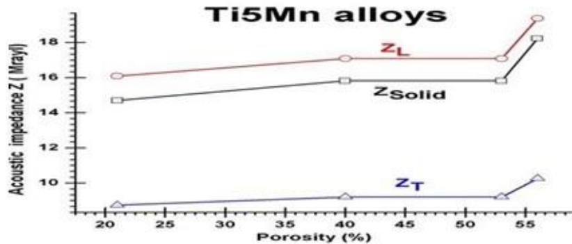
**FIG. 3. Characteristic Acoustic impedance of Porous Ti5Mn alloys, for a Solid Acoustic impedance Z<sub>Solid</sub> (—), Longitudinal Acoustic impedance Z<sub>L</sub> (—) and Transvers Acoustic impedance Z<sub>T</sub> (—).**
