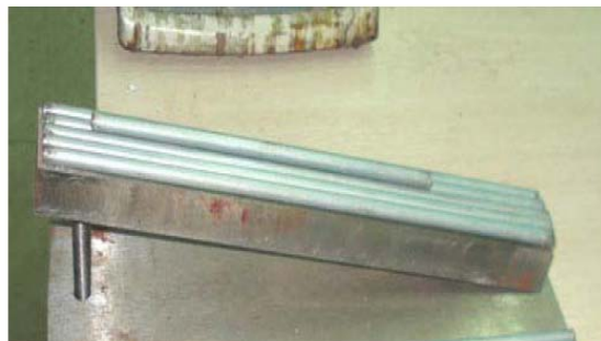
Figure 2: Friction coefficient test under the action of gravity
