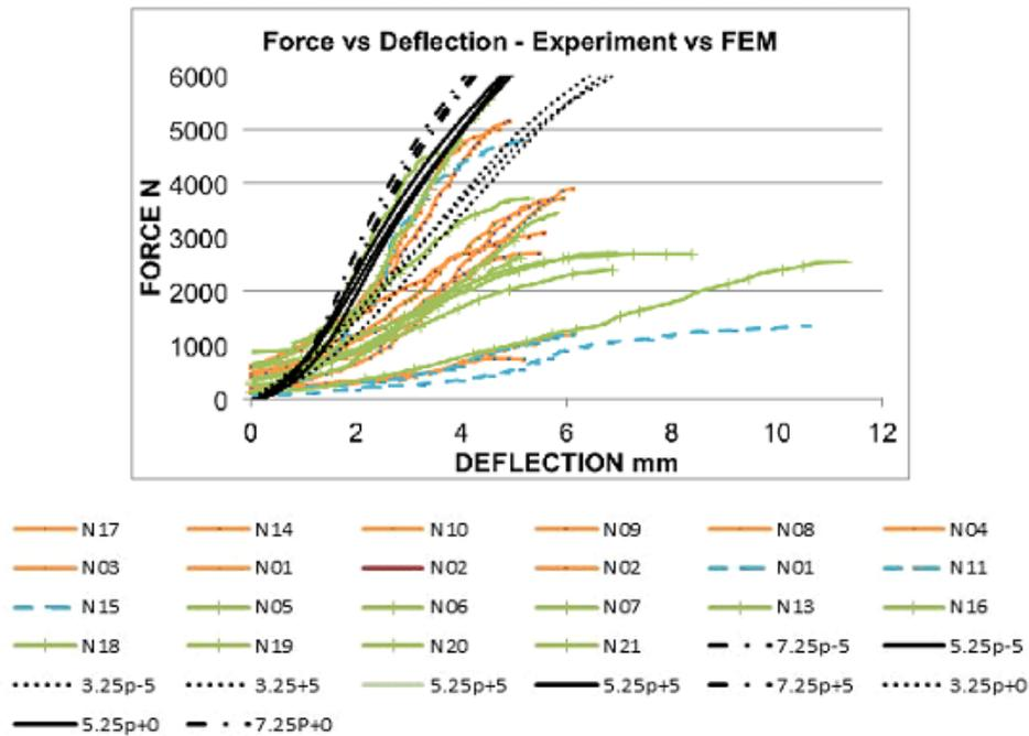
Figure 5 : Model predicted neck force-deflection vs experiment results in<sup>[6]</sup>.
