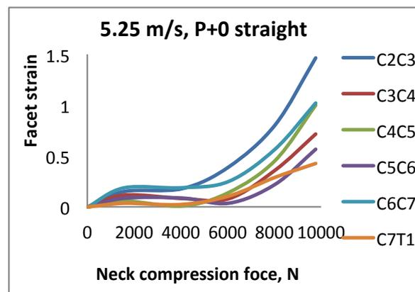
**Figure 6b : Facet resultant strain as the function of neck compression force with more sliding occurs in C2-C3 facet in straight neck position from 5.25 m/s impact.**
