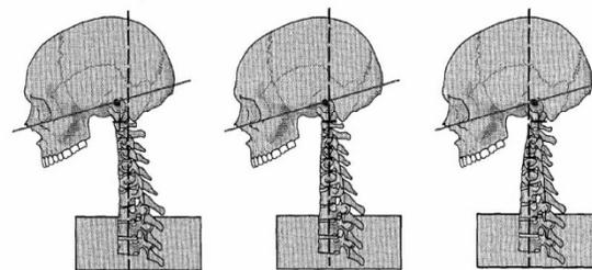
**Figure 1b : Experimental positions inducing flexion, compression and extension type injuries (Left: flexion position; Middle: stiff position; Right: extension position).**
