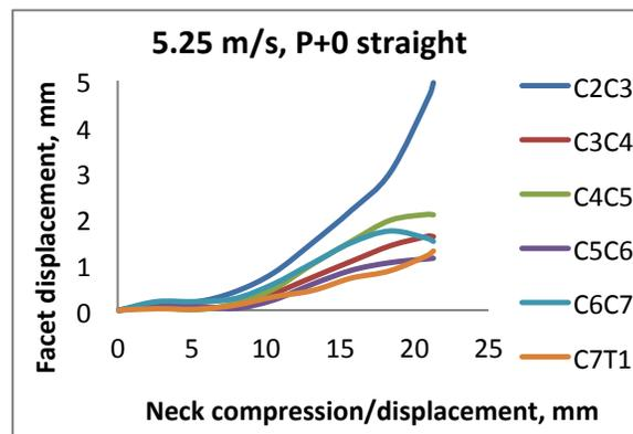
Figure 6a : Facet resultant displacement as the function of neck compression with more sliding occurs in C2-C3 facet in straight neck position from 5.25 m/s impact.
