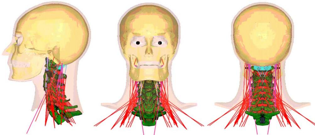
**Figure 3 : Integrated 50th percentile human head-neck model with various ligaments and joint capsule and muscles.**
