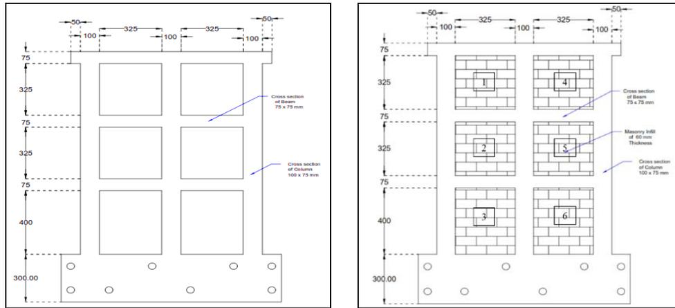
**Fig. 1: Bare frame details and infill frame details**
