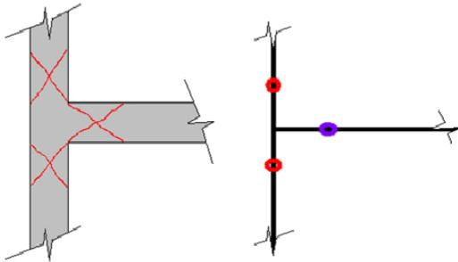
**Fig. 4: Location of hinges and crack formation**
