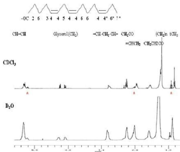
**Figure 1. (top) : proton nomenclature (middle trace) : <sup>1</sup>H-NMR (400.13MHz) spectrum of SSO (10 $\mu$ L/mL), 298K, in CDCl<sub>3</sub>. (bottom trace) : <sup>1</sup>H-NMR spectrum of SSO (10 $\mu$ L/mL) in D<sub>2</sub>O, 298K. The resonances specific of ( $\omega$ -3 chains are labeled with a star.**
