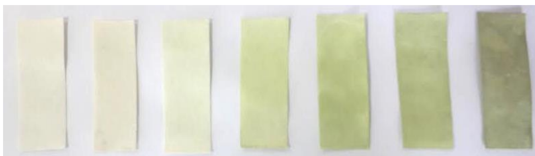
FIG. 8. Filter paper-based strips for the visual detection of presence Cu 2+ ion, 1. Receptor 1 and Cu(Ac) 2 deposited paper strips, 2. Paper strips dipped 1 mM of the CuCl 2 solution, 3. Paper strips dipped 2 mM of the CuCl 2 solution, 4. Paper strips dipped 4 mM of CuCl 2 solution (detectable colour change is observed), 5. Paper strips dipped 8 mM of the CuCl 2 solution, 6. Paper strips dipped 10 mM of the CuCl 2 solution, 7. Paper Strips dipped 25 mM of the CuCl 2 solution.
