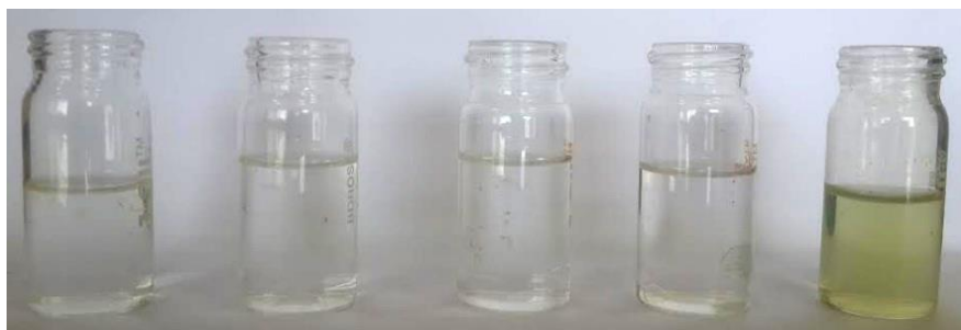
FIG. 2. 1. Receptor 1 (0.5 mM) in ethanol, 2. Mixing proper proportions of 1 (0.5 mM) and 1 mM \text{CuCl}_2 , 3. Receptor (0.5 mM) and 12.5 mM of \text{NaOAc} , 4. \text{NaOAc} (12.5 mM) and 1 mM \text{CuCl}_2 , 5. Receptor 1 (0.5 mM), 1 mM \text{CuCl}_2 and 12.5 mM of \text{NaOAc} .
