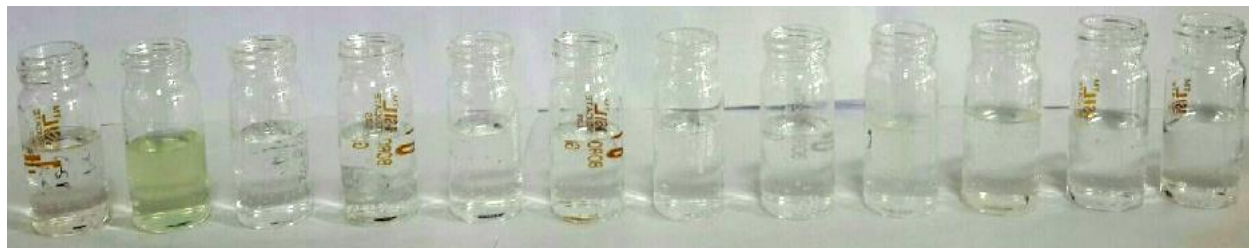
FIG. 5. Receptor 1 (0.5 mM), NaOAc (12.5 mM) and \text{MX}_2 (1 mM) are mixed in proper proportions. \text{CoCl}_2 , \text{CuCl}_2 (colour change observed), \text{MnCl}_2 , \text{BaCl}_2 , \text{KCl} , \text{SrCl}_2 , \text{AlCl}_3 , \text{HgCl}_2 , \text{CdCl}_2 , \text{LiCl} , \text{Pb}(\text{NO}_3)_2 .
