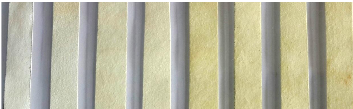
FIG. 14. Filter paper-based strips for the visual detection of presence Cu (II) ion, 1. Receptor 1 deposited paper strips, 2. Paper strips dipped 0. 2 mm of \text{CuCl}_2 solution 3. Paper strips dipped 0. 4 mm of the \text{CuCl}_2 solution, 4. Paper strips dipped 0.6 mm of \text{CuCl}_2 solution 5. Paper strips dipped 0. 8 mm of \text{CuCl}_2 solution (detectable colour change is observed) 6. Paper strips dipped 1.0 mm of the \text{CuCl}_2 solution. 7. Paper strips dipped 1.2 mm of \text{CuCl}_2 solution 8. Paper strips dipped 1. 4 mm of \text{CuCl}_2 solution.
