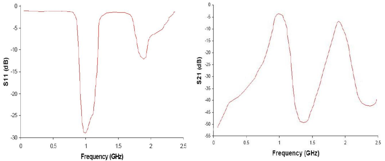
Figure 3 : Transmission and Reflection coefficients for zero iteration.
