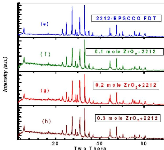
(e)  $x = 0.0$  mole (f)  $x = 0.1$  mole (g)  $x = 0.2$  mole (h)  $x = 0.3$  mole superconductors prepared by freeze drying technique.
