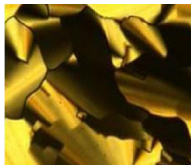
Highly ordered smectic-B phase at temperature 65 °C (250X)
