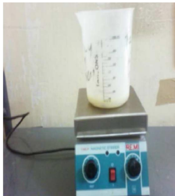
Figure 2 : Mixing of MQL and AL_2O_3 nanoparticles using magnetic stirrer
