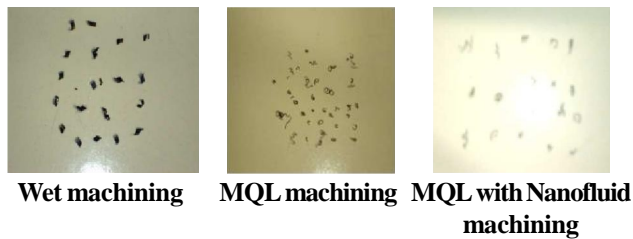
Figure 6 : Actual forms of chips produced during turning at optimal level of cutting parameter under (a) wet, (b) MQL and (c) MQL with Nanofluid conditions
