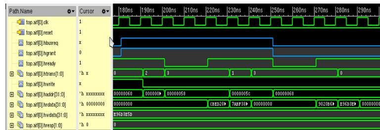
Fig. 6: INCR 4 read test case
