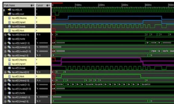
Fig. 7: Locked transfer test case
