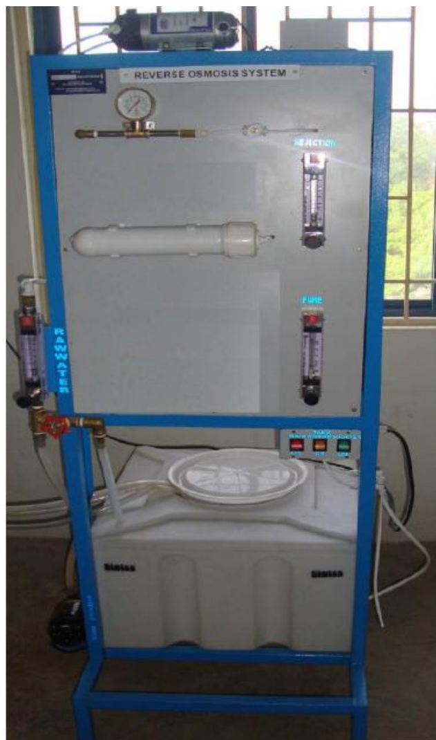
Figure 1 : Picture of reverse osmosis (RO) unit
