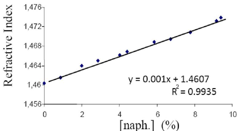
Figure 1 : Calibration curve fuel-naphthalene []
