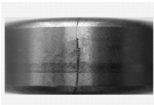
Figure 7. Schematic diagram of bearing outer crack fault
