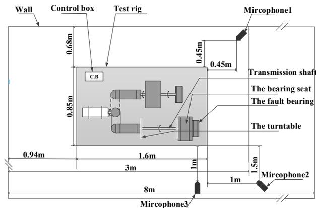
**Figure 3. The position chart of test-rig and microphones**
