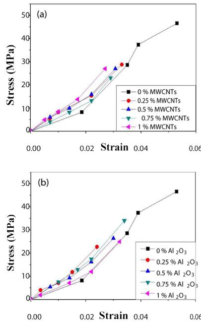
FIG. 6. Stress strain behavior for (a) Epoxy/MWCNTs and (b) Epoxy/Al<sub>2</sub>O<sub>3</sub> nanocomposites.
