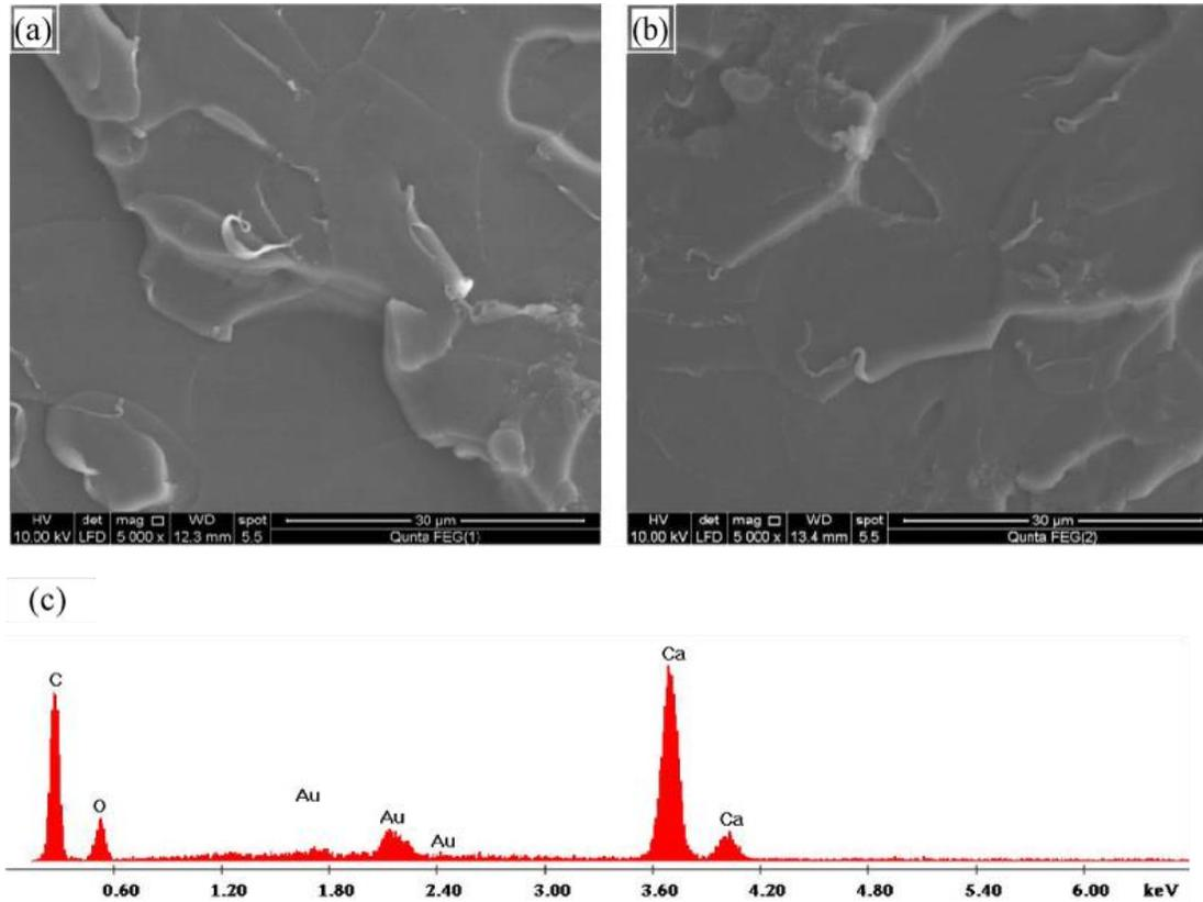
FIG. 10. SEM images of the fracture surface after tensile test of (a) Epoxy/0.25 MWCNTs, (b) Epoxy/1 MWCNTs nanocomposite and (c) EDS spectrum of Epoxy/MWCNTs nanocomposites.
