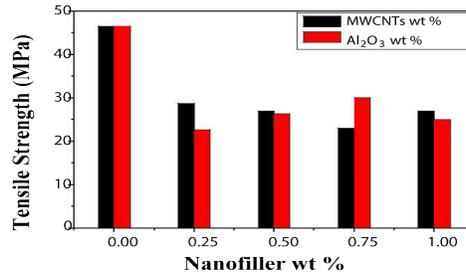
FIG. 5. Average values of ultimate tensile strength for Epoxy/MWCNTs and Epoxy/Al<sub>2</sub>O<sub>3</sub> nanocomposites.
