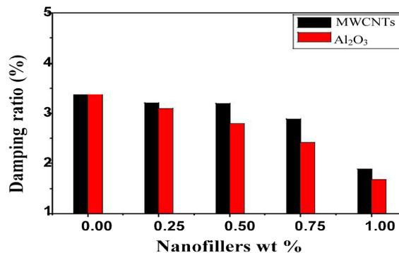
FIG. 13. Damping ratio for Epoxy/MWCNTs and Epoxy/ $\text{Al}_2\text{O}_3$  nanocomposites.
