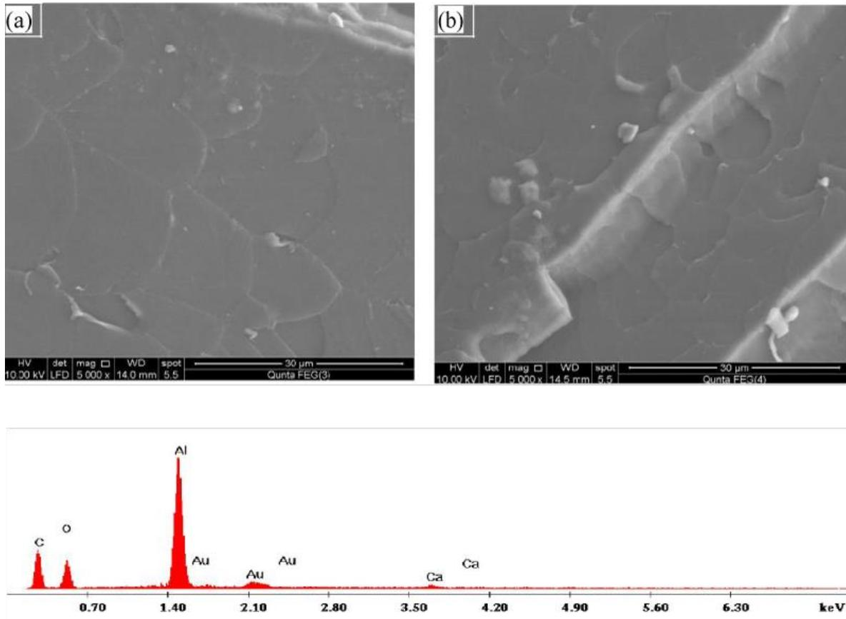
FIG. 11. SEM images of the fracture surface after tensile test of (a) Epoxy/0.25  $\text{Al}_2\text{O}_3$ , (b) Epoxy/1  $\text{Al}_2\text{O}_3$  nanocomposite and (c) EDS spectrum of Epoxy/ $\text{Al}_2\text{O}_3$  nanocomposites.
