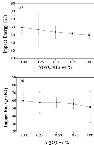
FIG. 7. The Impact energy of (a) Epoxy/MWCNTs and (b) Epoxy/ $\text{Al}_2\text{O}_3$  nanocomposites.
