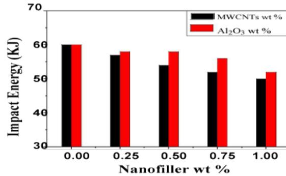
FIG. 8. The average values of impact energy for Epoxy/MWCNTs and Epoxy/Al<sub>2</sub>O<sub>3</sub> nanocomposites.
