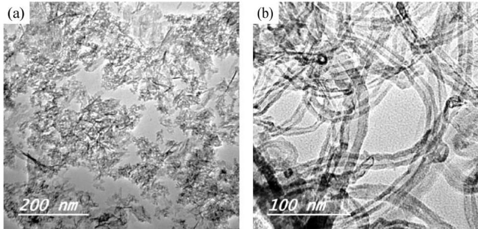
FIG. 2. TEM micrographs of raw material (a) Al<sub>2</sub>O<sub>3</sub> nanoparticles and (b) MWCNTs.
