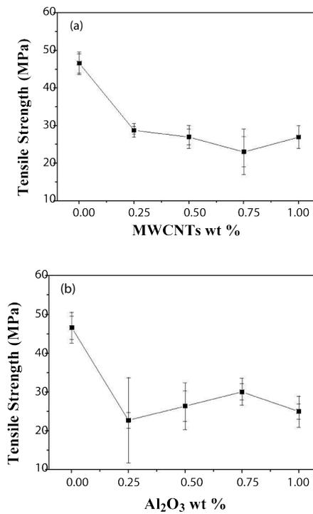
FIG. 4. The ultimate tensile strength of (a) Epoxy/MWCNTs and (b) Epoxy/Al<sub>2</sub>O<sub>3</sub> nanocomposites.
