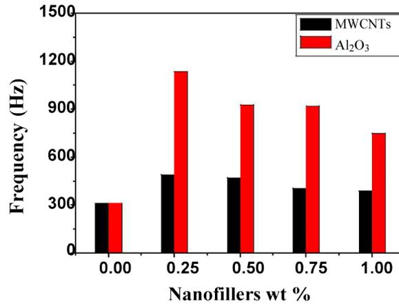
FIG. 12. Frequency response for Epoxy/MWCNTs and Epoxy/ $\text{Al}_2\text{O}_3$  nanocomposites.
