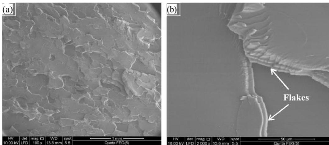
FIG. 9. SEM images of the fracture surface after tensile test of neat Epoxy (a) 100X (b) 2000X.
