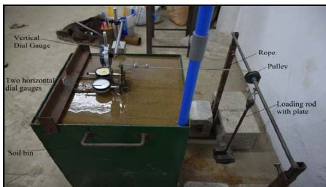
Fig. 2: Horizontal loading arrangement
