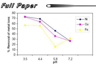
Figure 1 : Effect of pH on removal of metal ions
