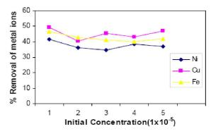
Figure 3 : Effect of initial concentration on removal of metal ions
