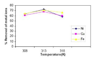
Figure 4 : Effect of temperature on removal of metal ions
