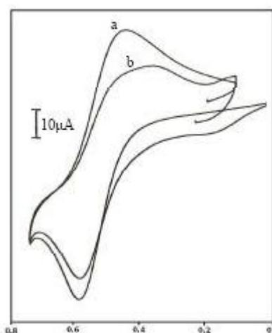
Figure 6: Cyclic voltammograms of 1mM  $\text{Cu}(\text{HAO})_2\text{Py}_2$  complex (a) in absence of CT DNA and (b) in presence of CT DNA (5  $\mu\text{M}$ ) at scan rates
