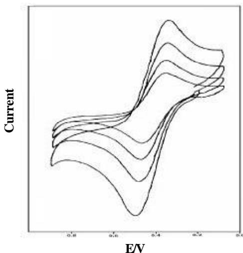
Figure 4: Cyclic voltammetry of [Cu(HAO)<sub>2</sub>Im<sub>2</sub>], at repeated scans at different scan rates 25, 50, 100 and 200 mVs<sup>-1</sup>
