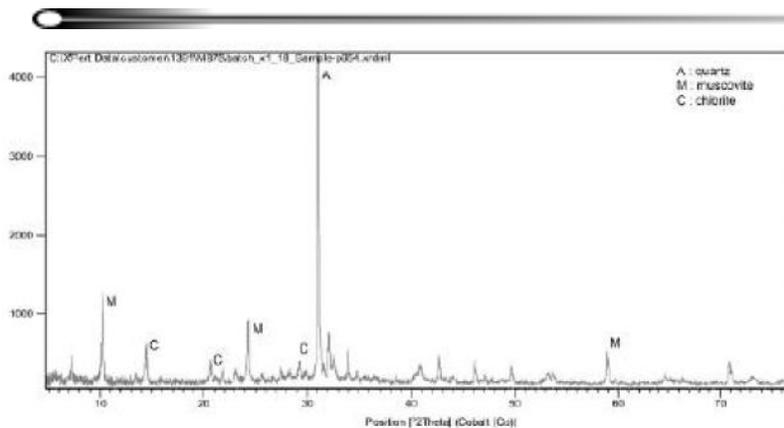
Figure 2 : The XRD image of the waste
