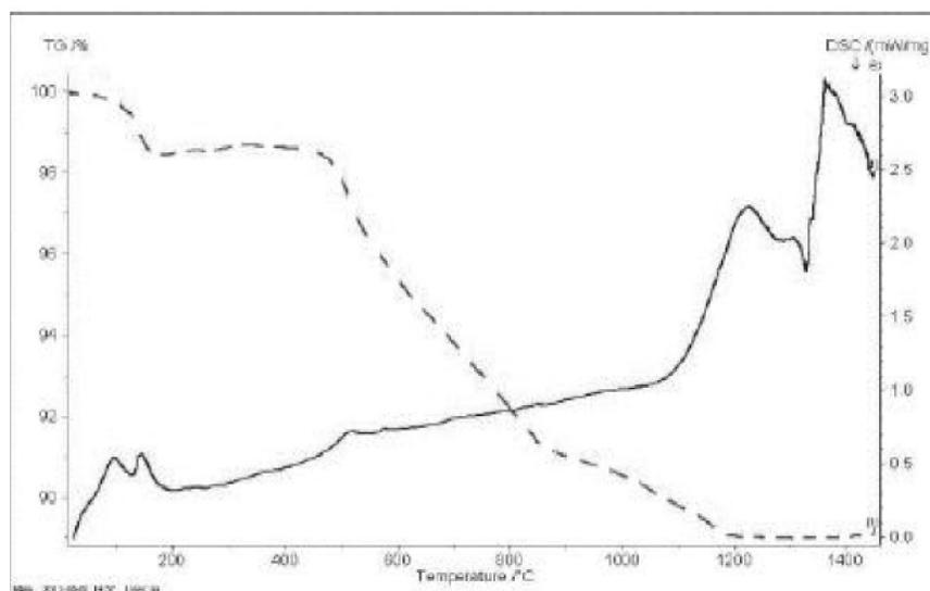
Figure 6 : TG and DSC curves of the waste
