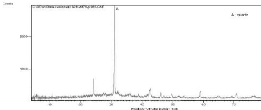
Figure 3 : The XRD image of the sintered single soil sample of W
