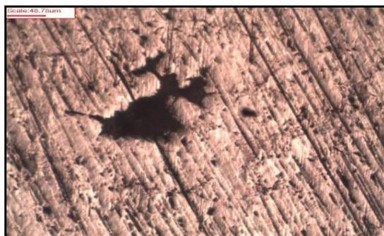
**Fig. 7: Aluminium Alloy 5083 micro structure after immersion test**
