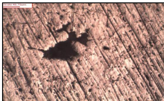
Fig. 7: Aluminium Alloy 5083 micro structure after immersion test
