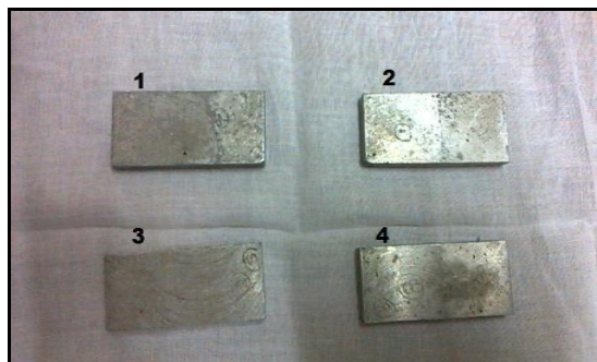
Fig. 6: Specimens after immersion test at 200°C
