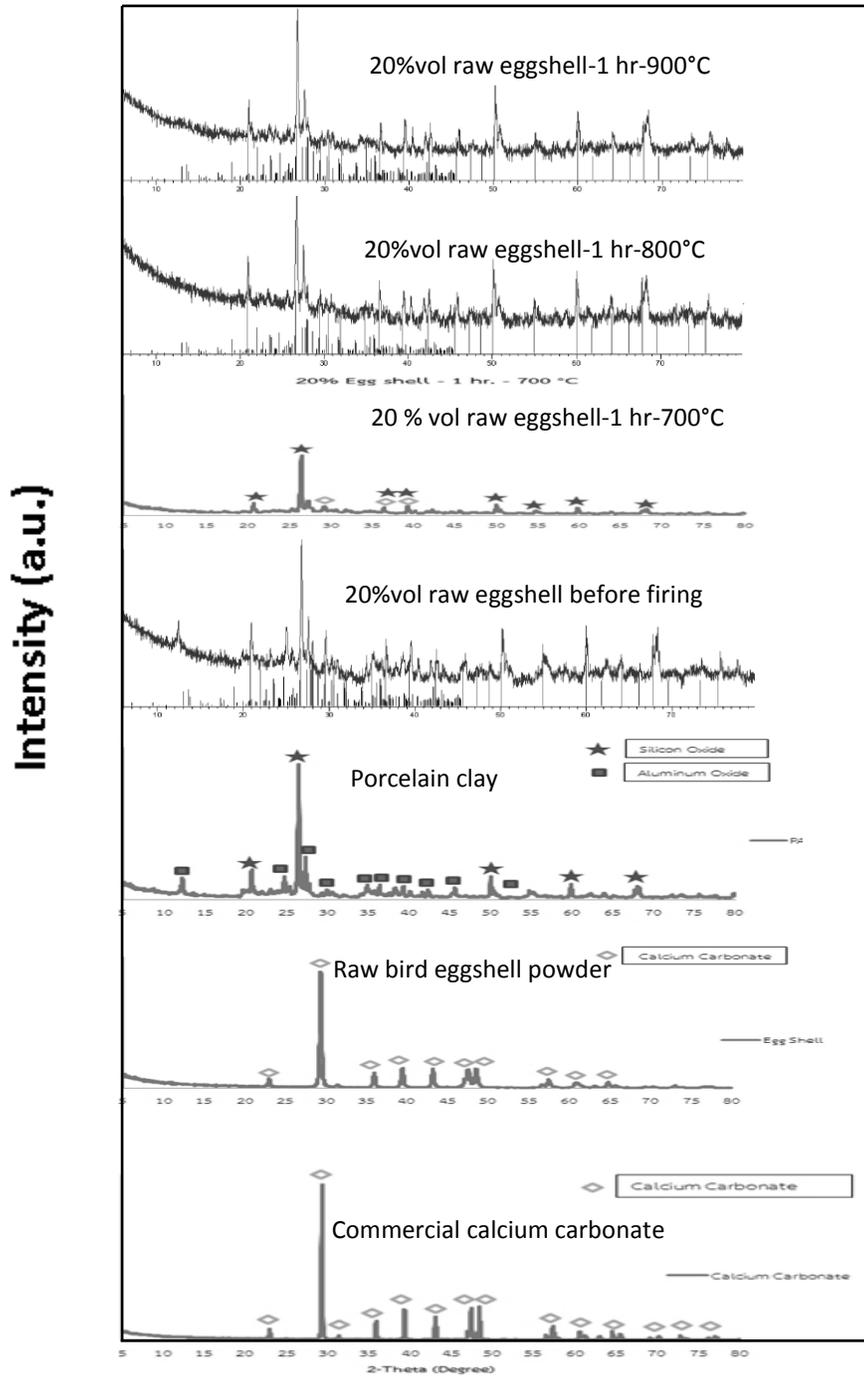
FIG. 2. X-ray patterns of raw bird eggshell powder, porcelain clay, and porcelain products added raw bird eggshell powder before/after firing.
