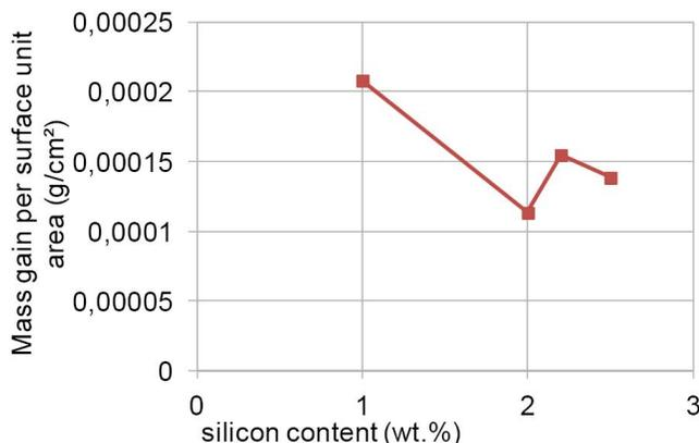
**Figure 6 :** Evolution of the mass gain observed at the end of the first linear oxidation part
