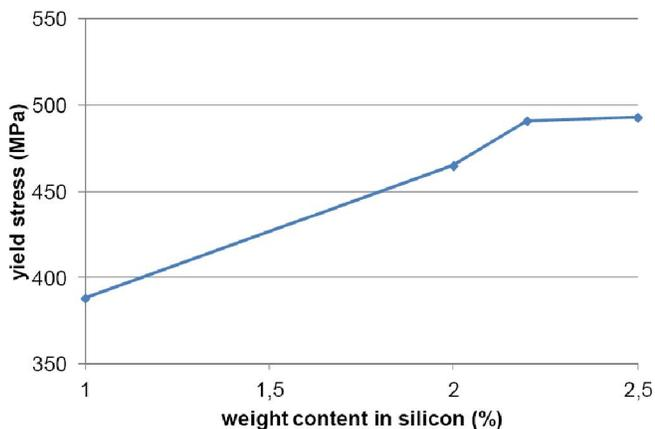
**Figure 2 : Evolution of the yield stress versus the silicon content in the steel**
