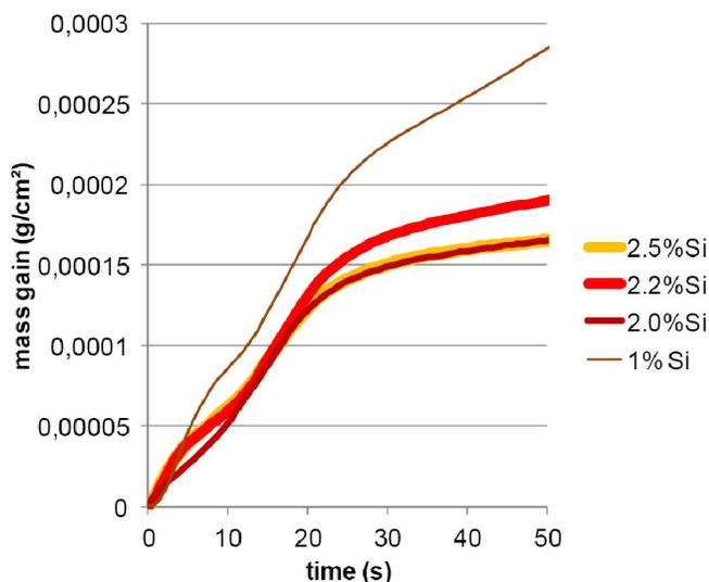
**Figure 5 :** Mass gain curves obtained for the four steels (zoomed on the linear first part)
