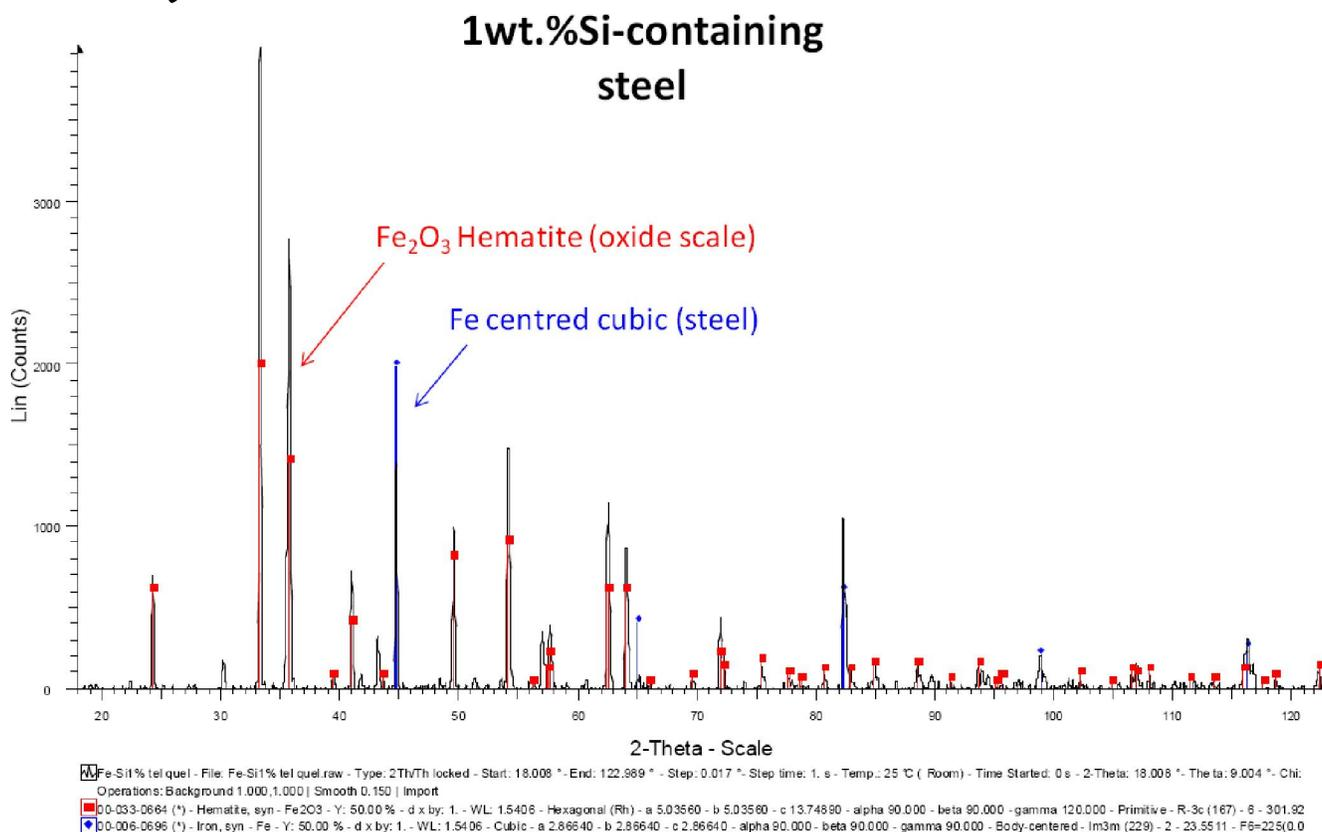
Figure 8 : The XRD Spectra acquired on the oxidized surface of the 1wt.%Si-containing steel
