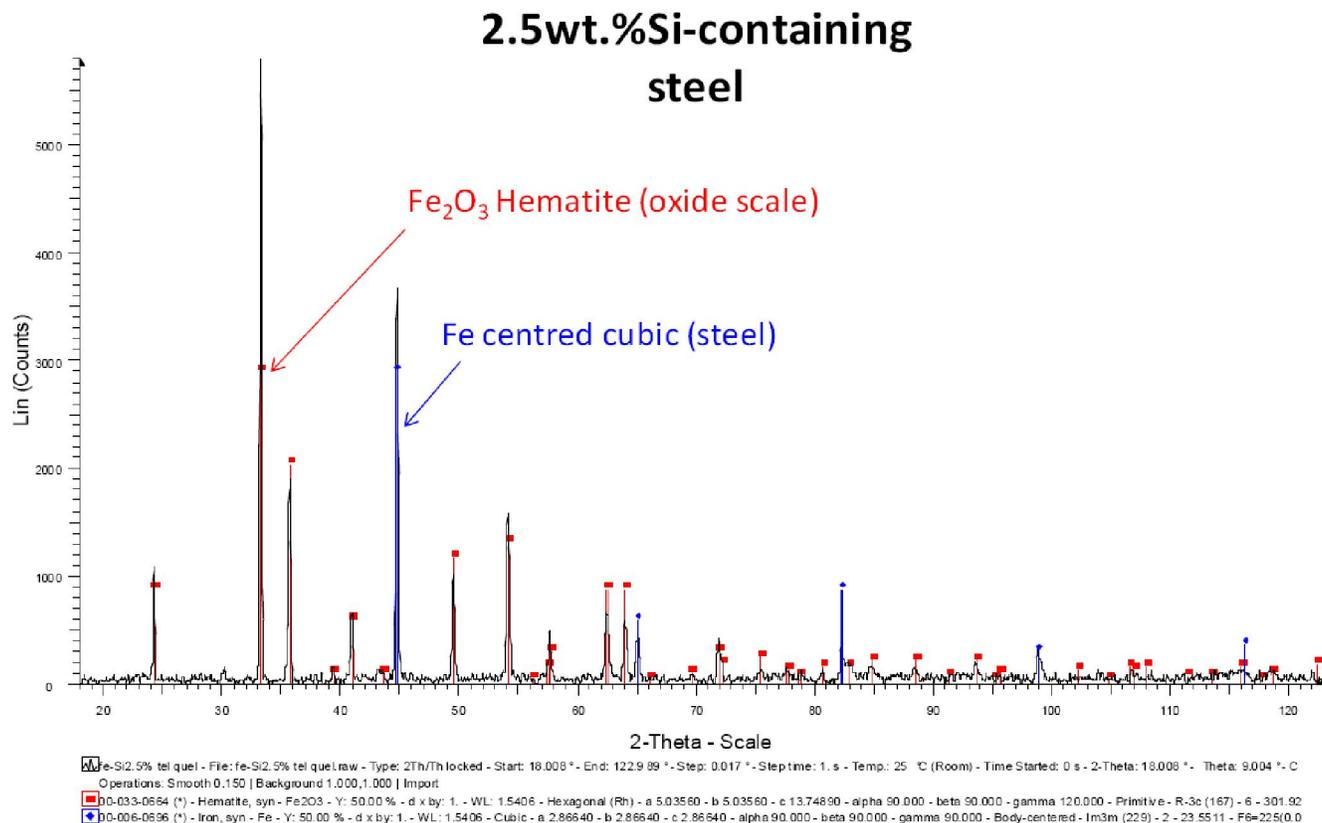
Figure 9 : The XRD Spectra acquired on the oxidized surface of the 2.5wt.%Si-containing steel
