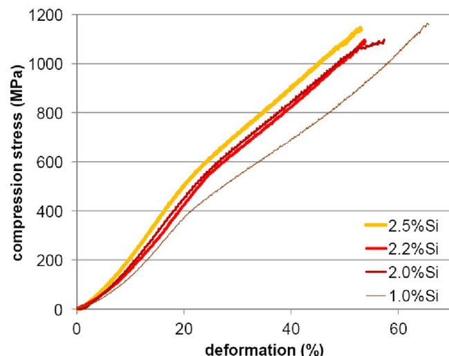
Figure 1 : Strain-stress curves acquired during the compression tests applied to the four steels
