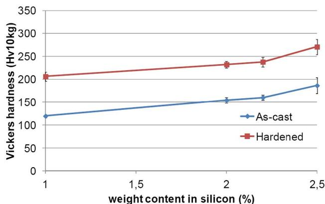
**Figure 3 : Curves of hardness variation illustrating the strengthening and hardening effects of the silicon content and of the compression tests**
