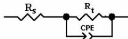
Figure 4 : Equivalent circuit used to represent the impedance result without and with inhibitor
