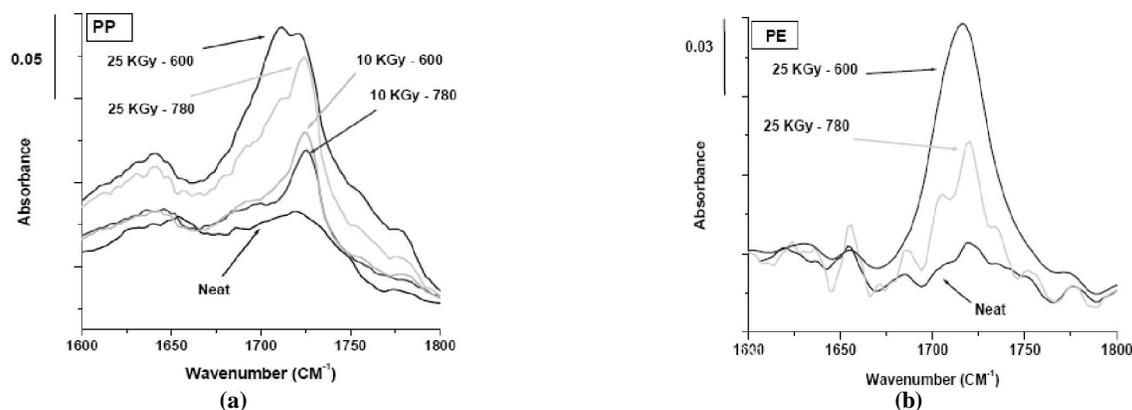
Figure 2 : FTIR spectra of neat and  $\gamma$ -sterilized (a) PP and (b) PE at carbonyl region with different dose rate
