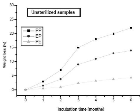
Figure 5 : Weight loss (%) of unsterilized samples
