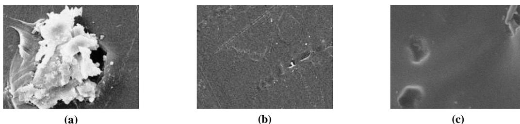
Figure 8 : SEM of  $\gamma$ -sterilized (with dose rate  $780 \text{ Gyh}^{-1}$  and 4 months composted samples (a) PP, (b) PE, and (c) EP
