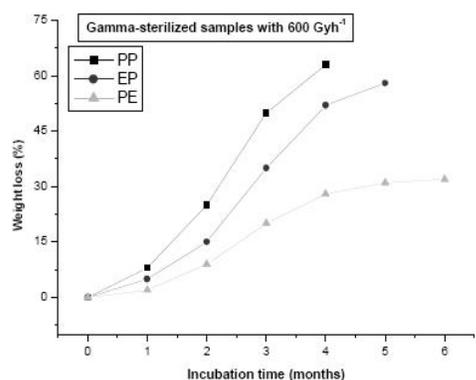
Figure 6 : Weight loss (%)  $\gamma$ -sterilized samples with dose rate  $780 \text{ Gyh}^{-1}$
