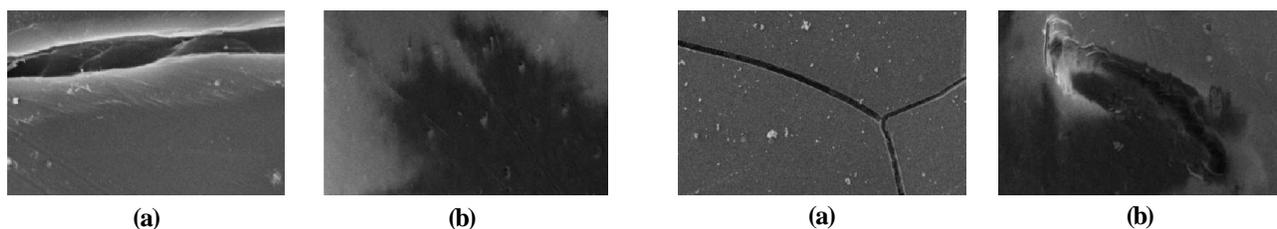
Figure 3 : SEM of  $\gamma$ -sterilized samples (with dose rate 780  $\text{Gyh}^{-1}$ ) a) PP and b) PE
