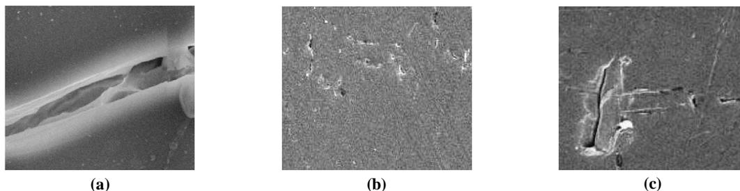
Figure 9 : SEM of  $\gamma$ -sterilized (with dose rate  $600 \text{ Gyh}^{-1}$ ) and 4 months composted samples (a) PP (b) PE and (c) E
