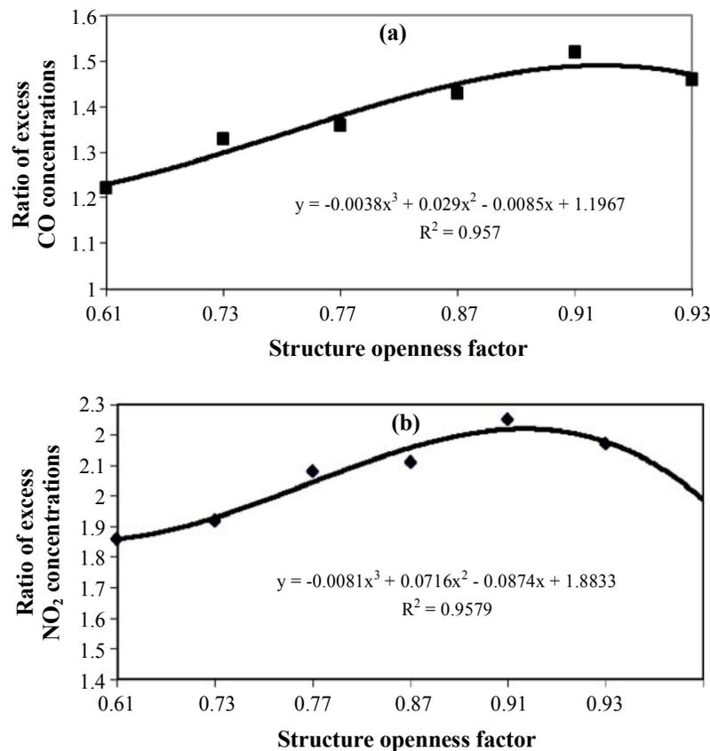
**Fig. 1: Relationship between the ratio of excess concentrations at distances of 1 m to 100 m and the openness factor: (a) carbon oxide CO, (b) nitrogen dioxide NO<sub>2</sub>**
