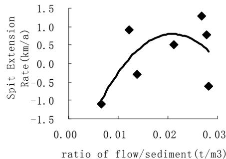
Figure 4 : Relationship Curve between the Spit Extension Rate and Flow/Sediment
