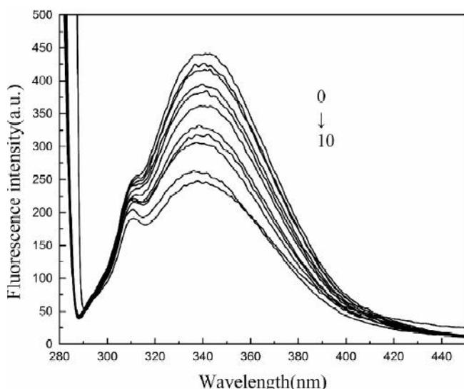
**Figure 2 :** Fluorescence spectra of BSA-PGH system ( $T = 298 \text{ K}$ ,  $\lambda_{ex} = 280 \text{ nm}$ );  $C_{BSA} = 2.0 \times 10^{-7} \text{ mol} \cdot \text{L}^{-1}$ ,  $0 \sim 10 C_{PGH} = (0, 0.5, 2.0, 3.0, 4.0, 5.0, 7.0, 8.0, 10.0, 15.0, 20.0) \times 10^{-5} \text{ mol} \cdot \text{L}^{-1}$
