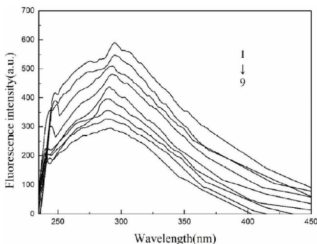
Figure 3 : Elastic scattering fluorescence spectra of BSA-PGH system ( $T = 298 \text{ K}$ );  $C_{\text{PGH}} = 2.5\times 10^{-5} \text{ mol}\cdot\text{L}^{-1}$ ,  $1\sim 9C_{\text{BSA}} = (0, 1.0, 1.5, 2.0, 2.5, 3.0, 3.5, 4.0, 4.5) \times 10^{-7} \text{ mol}\cdot\text{L}^{-1}$
