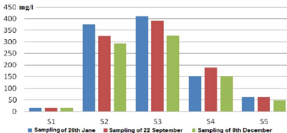
Figure 6 : Evolution of the BOD5 in the water during three sampling periods
