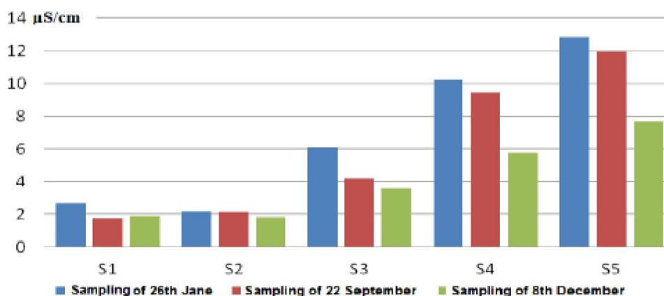
Figure 4 : Evolution of the electrical conductivity in the water during three sampling periods
