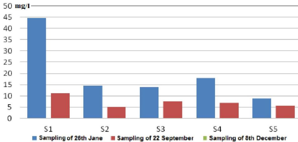
Figure 8 : Evolution of the Nitrate concentration in the water during three sampling periods
