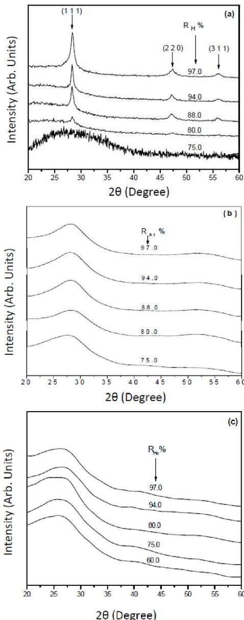
**Figure 3:** X-ray patterns of films deposited at different dilution of silane using different diluents (a) Hydrogen dilution of silane (b) Argon dilution of silane and (c) Helium dilution of silane.
