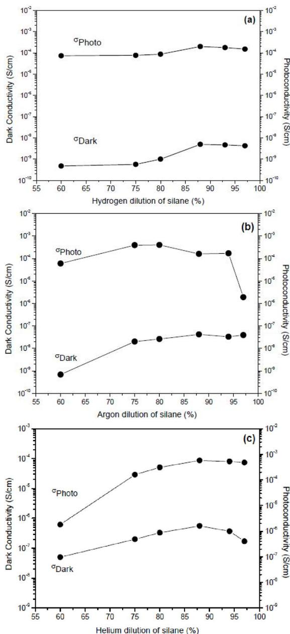
**Figure 6 :** Variation of dark and photoconductivity as a function of dilution of silane using different diluents for the nc-Si:H deposited thin films by HW-CVD.
