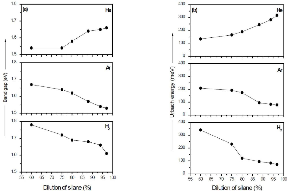
Figure 5: Variation of band gap and Urbach energy as a function of dilution of silane using different diluents for the nc-Si:H deposited thin films by HW-CVD.
