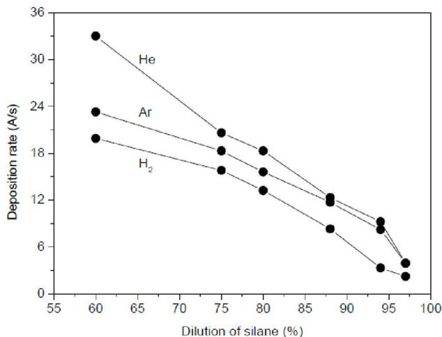
Figure 1 : Variation of deposition rate as a function of dilution of silane by  $\text{H}_2$ , Ar and He gases.
