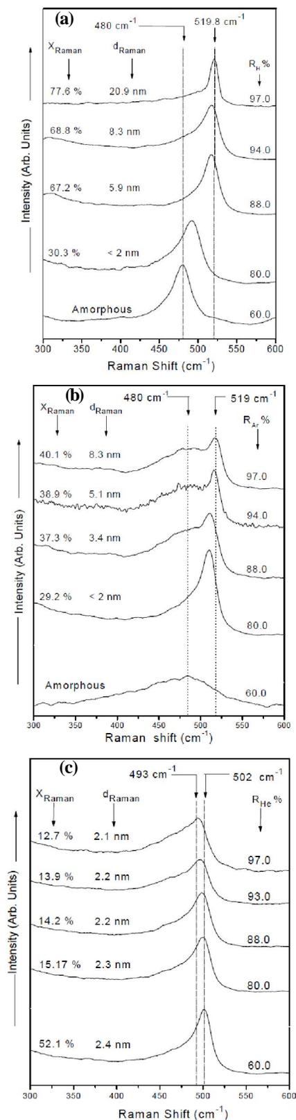
**Figure 2:** Raman spectra of films deposited at different dilution of silane using different diluents (a) Hydrogen dilution of silane (b) Argon dilution of silane and (c) Helium dilution of silane.
