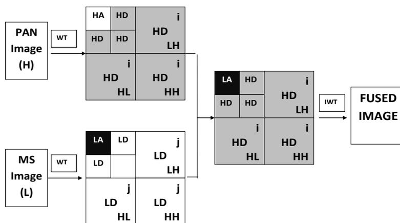
Fig. 1: Wavelet based fusion of multispectral and panchromatic images
