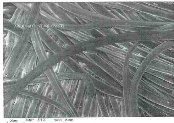
Figure 1: SEM of the unaffected control area of the garment
