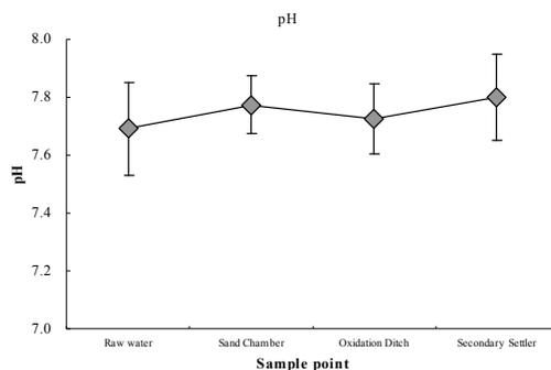
Figure 3 : Variation of pH in different stages in WWTP
