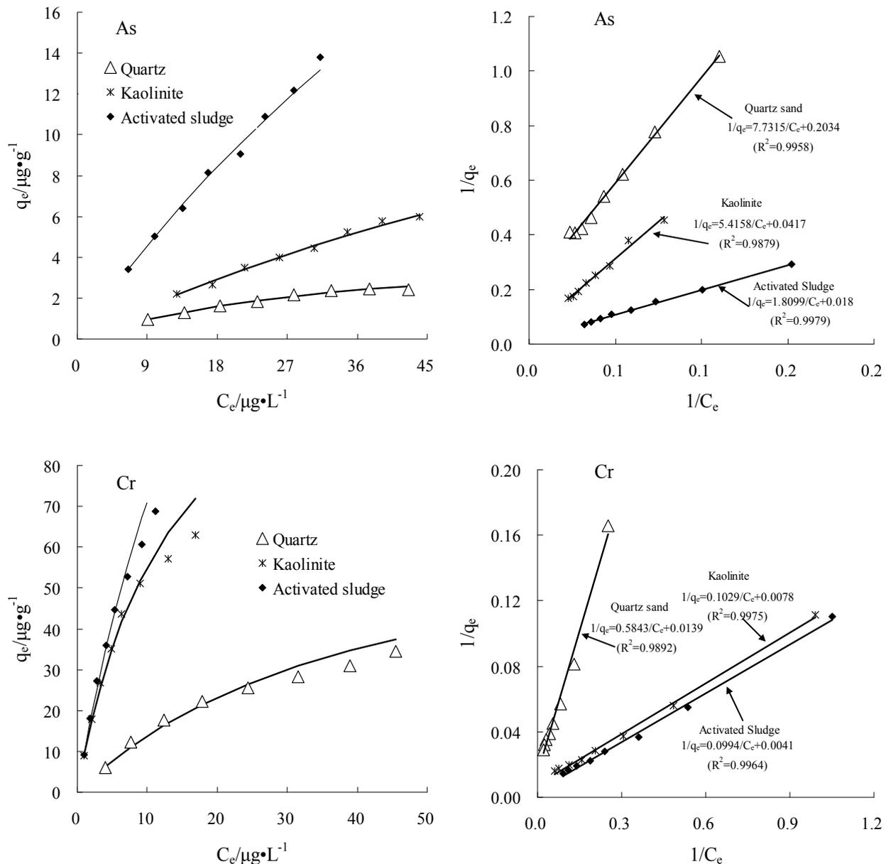
Figure 7 : Adsorption isotherms for As and Cr using the three types of adsorbent. Temperature =25°C, pH=6.0, mixing speed=160 rpm, adsorbent concentration=1000mg·L<sup>-1</sup> MLSS, solution volume=100mL, contact time=24h.
