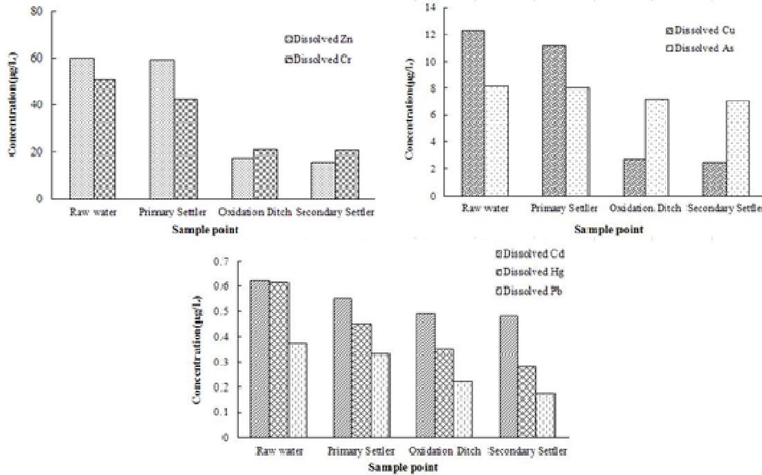
Figure 4 : Average distribution of the dissolved Cu, Zn, Pb, Cd, Hg and As in the different stages
