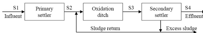
**Figure 1 : Schematic flow diagram and sampling point of the WWTP**
