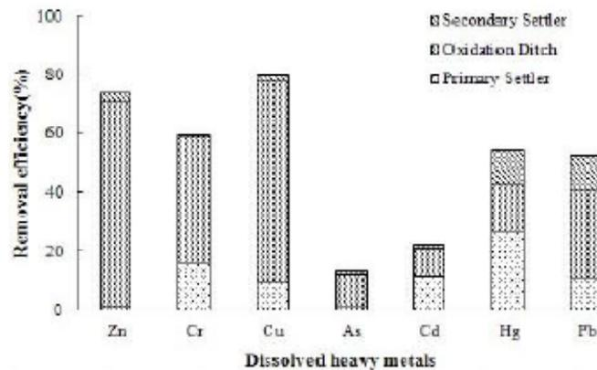
Figure 5 : Separate removal efficiency of the dissolved heavy metals
