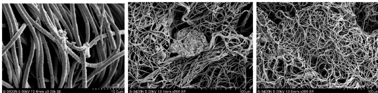
Figure 2 : SEM image of the activated sludge
