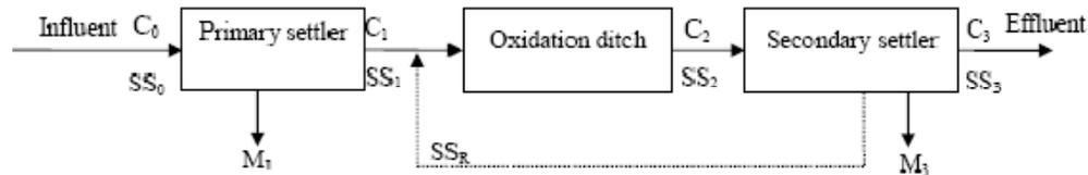
Figure 6 : Material balance along the WWTP
