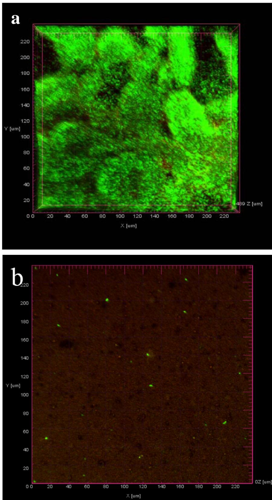
**Figure 4 :** Biofilm growth of *P. aeruginosa* PAO1 on control glass surface (a) and silver-embedded-coating (b). Attachment and biofilm growth was negligible on glass slides with silver-embedded coating. Control biofilm image was reconstructed with 16 xy-slices collected at a z-interval of 2 microns.
