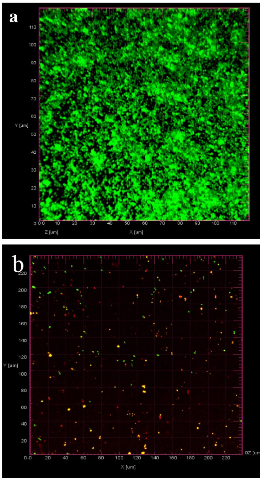
Figure 5 : Biofilm growth of *Staphylococcus aureus* on control (a) and silver-nanoparticle-embedded composite coated (b) glass surfaces. *S. aureus* colonization and biofilm growth was inhibited on glass slides with silver-embedded coating. The control biofilm image was reconstructed with 14 xy-slices collected at z-interval of 2 microns.
