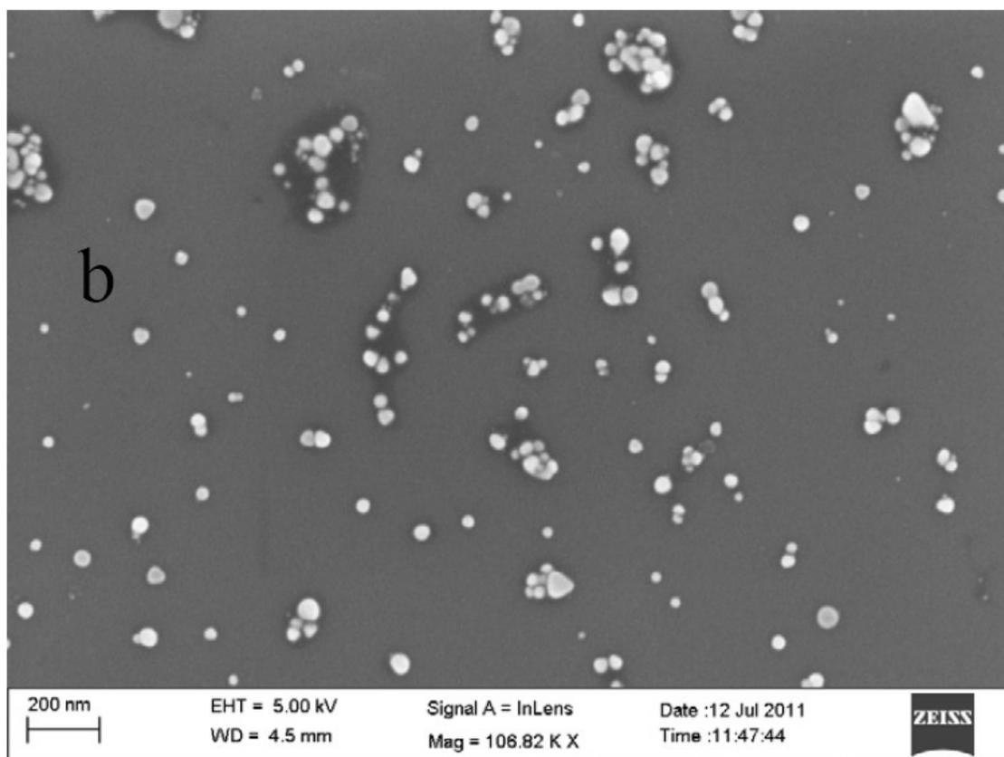
Figure 3 : UV-Vis spectra (a) and field-emission scanning electron microscope image (b) of silver-nanoparticle embedded coating.
