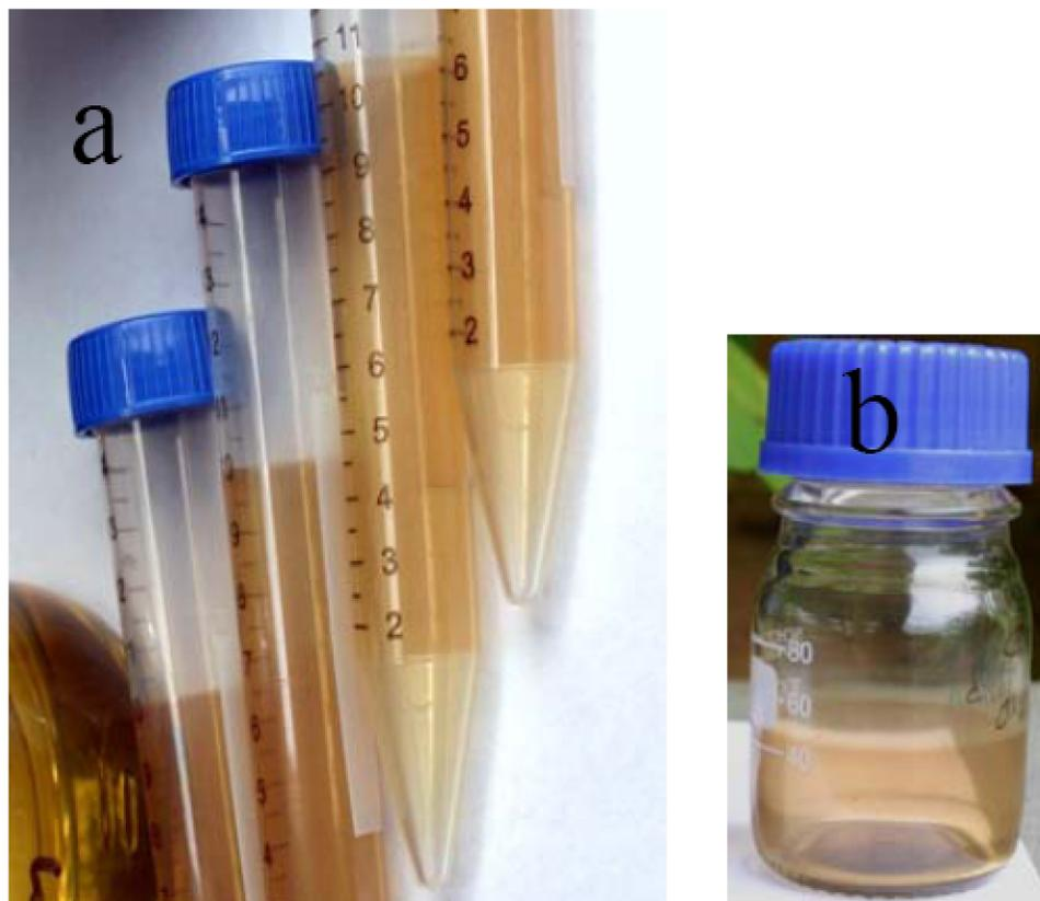
**Figure 2 :** Images of silver-nanoparticle-embedded coatings formed on polyvinyl chloride (a) and glass (b) surfaces. Yellow color indicates the deposition of silver-nanoparticle-embedded rosin composite.
