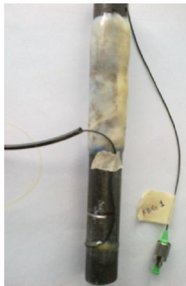
Figure 3 : FBG instrumented rebar
