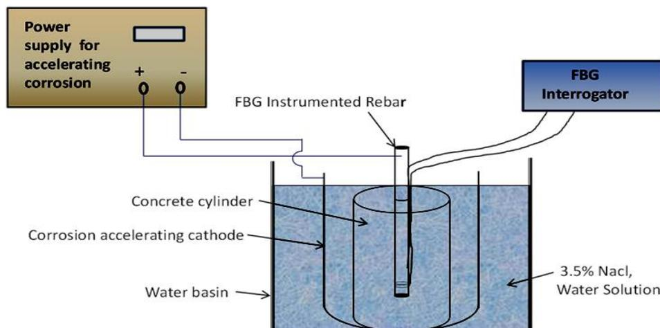
Figure 6 : Schematic illustration of accelerated corrosion test set up
