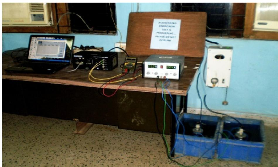
Figure 5 : Accelerated corrosion test set up
