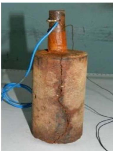
Figure 7 : Concrete specimen after cracking
