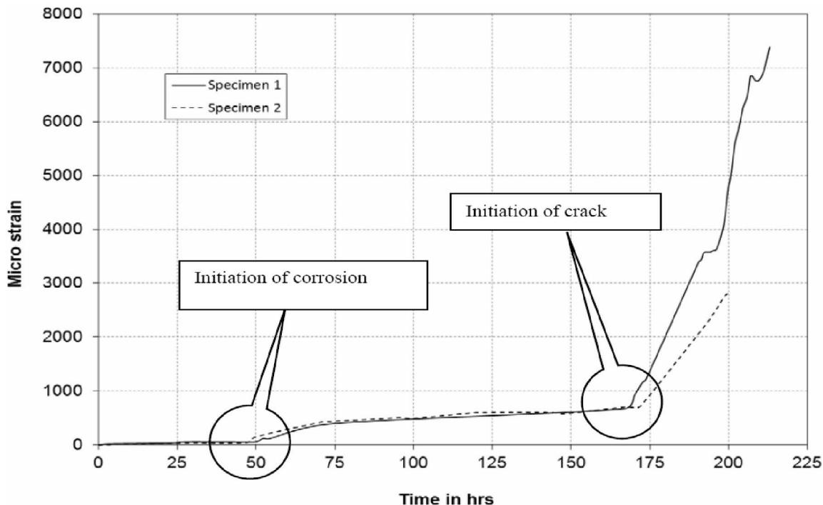
Figure 8 : Strain v/s time graph for specimens 1 and 2
