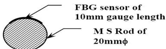
Figure 2 : Cross sectional view of the instrumented rebar
