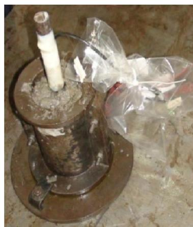
Figure 4 : Embedding of FBG instrumented rebar
