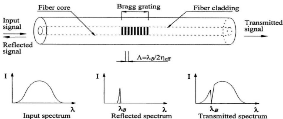
Figure 1 : Light spectra of a Fiber Bragg Grating sensor
