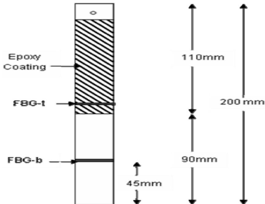
Figure 9 : Instrumentation details of MS rod for verification of methodology
