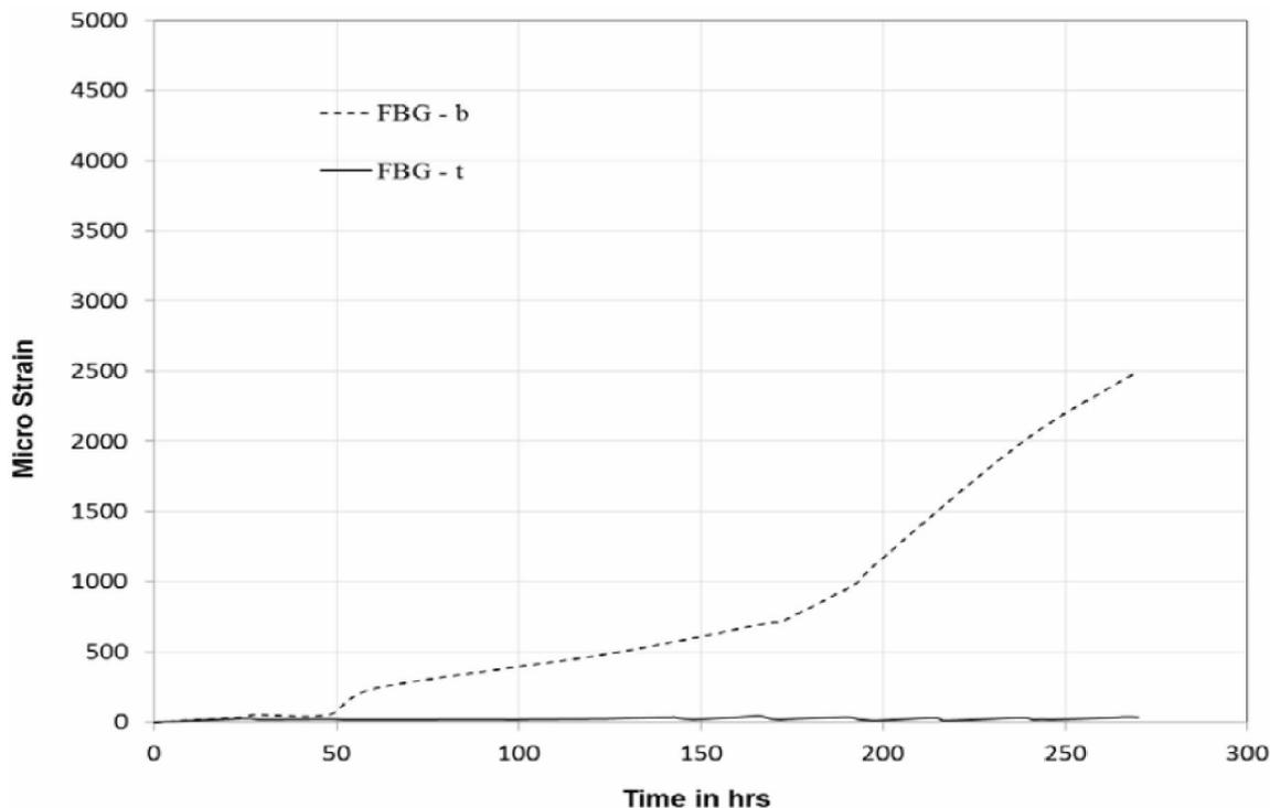
Figure 10 : Typical strain vs time graph from verification test
