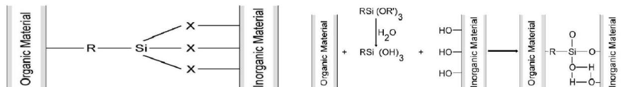
Figure 1 : Coupling mechanism of nanoparticles by organic silane
