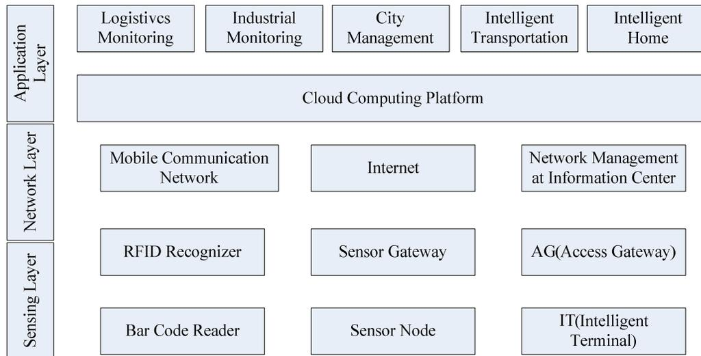
**Figure 2 : The Internet of things system architecture diagram**
