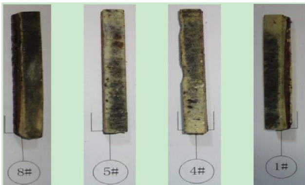
Figure 3 : The adhesion conditions of honing oilstone.
