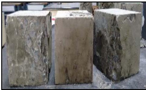
Fig. 4: 0.25% RFRC after testing
