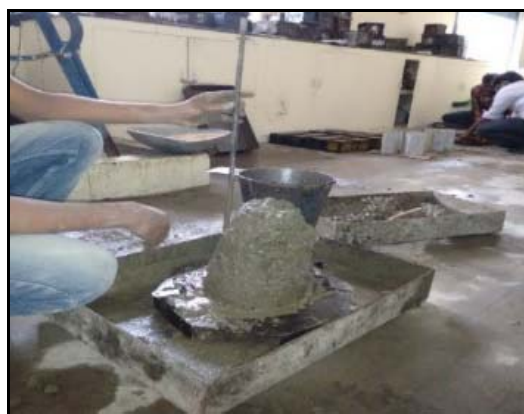
Fig. 3: Slump of RFRC
