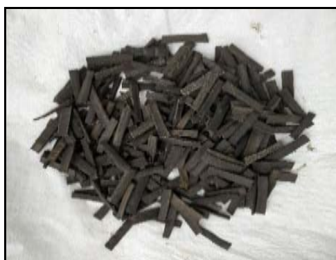
Fig. 1: Hand shredded cycle tyre
