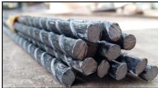
**Fig. 1: GFRP Bar**
