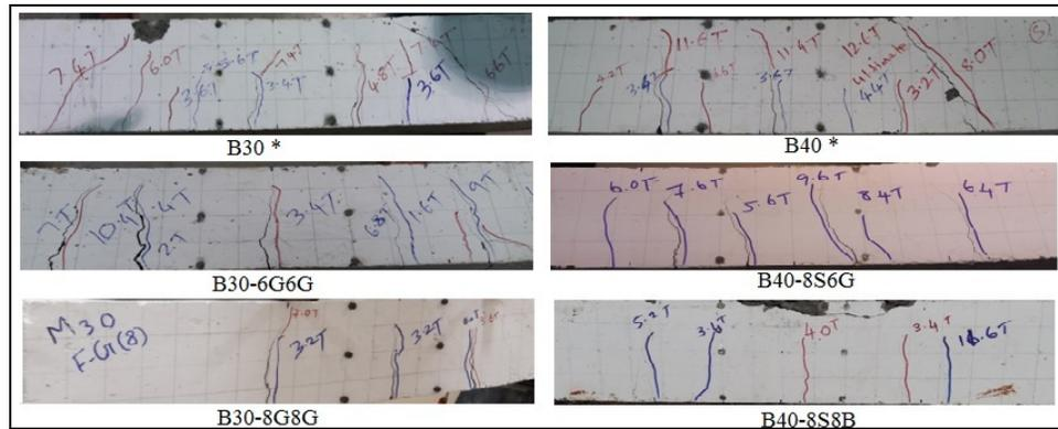
**Fig. 3: Crack pattern**
