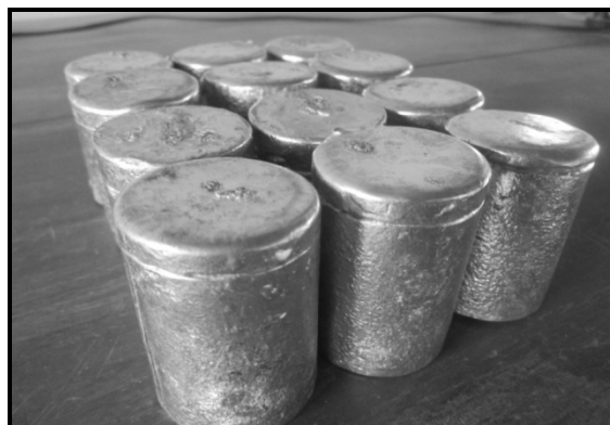
Fig. 1: Tin alloy (Matrix phase)
