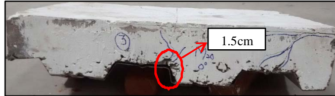
Fig. 10: Slip behaviour for slab 0^\circ
