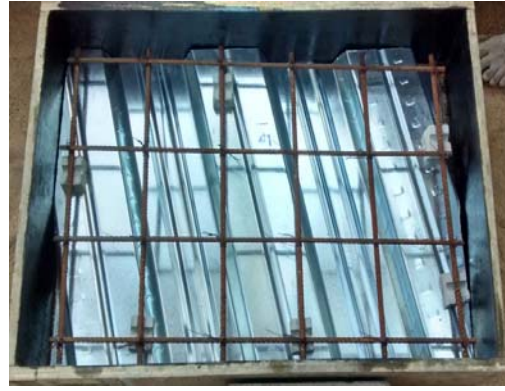
Fig. 2: Photograph of 15° profiled steel deck slab
