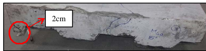
Fig. 11: Slip behaviour for slab 15^\circ
