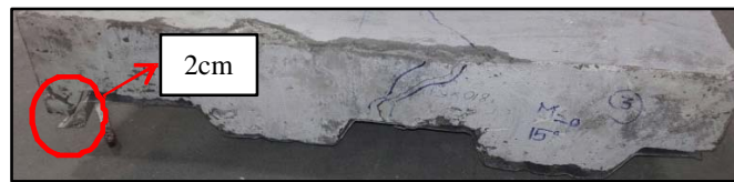
Fig. 11: Slip behaviour for slab 15°
