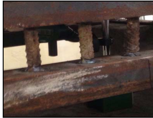
Fig. 7: Deflection transducer location during testing
