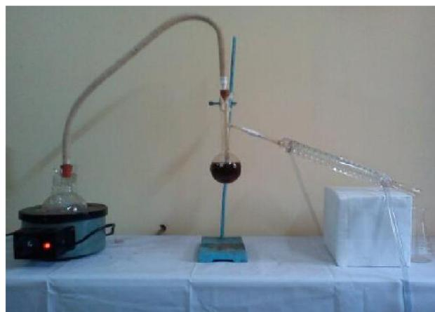
Figure 2 : Steam distillation apparatus
