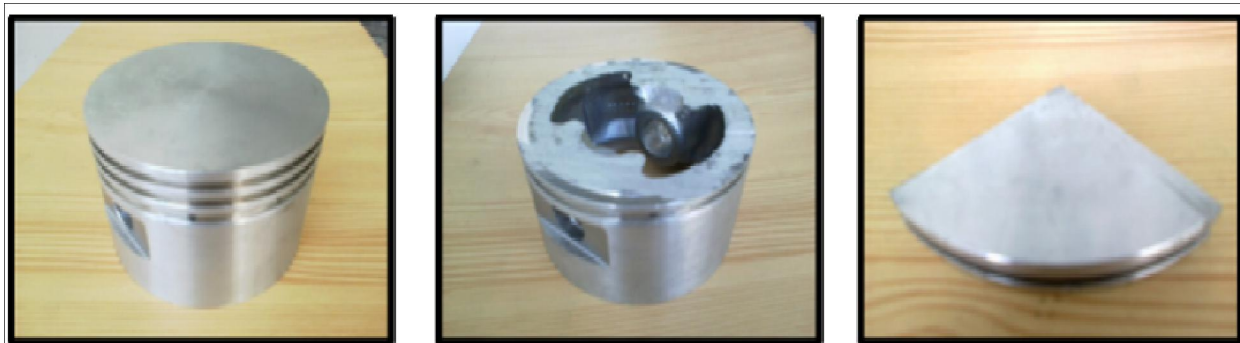
Figure 1 : Flat top surface piston (left); piston after top portion removal (middle) and 5 mm thick quarter portion specimen (right)
