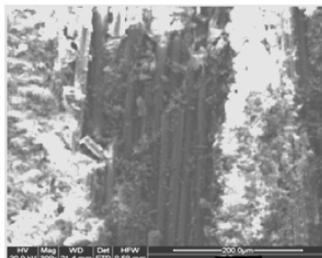
**Figure 6(b) : SEM of (GV<sub>2</sub>) at load 30N & speed 2m/s**
