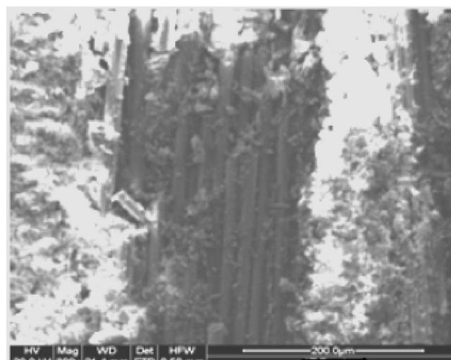
**Figure 6(b) : SEM of (GV<sub>2</sub>) at load 30N & speed 2m/s**
