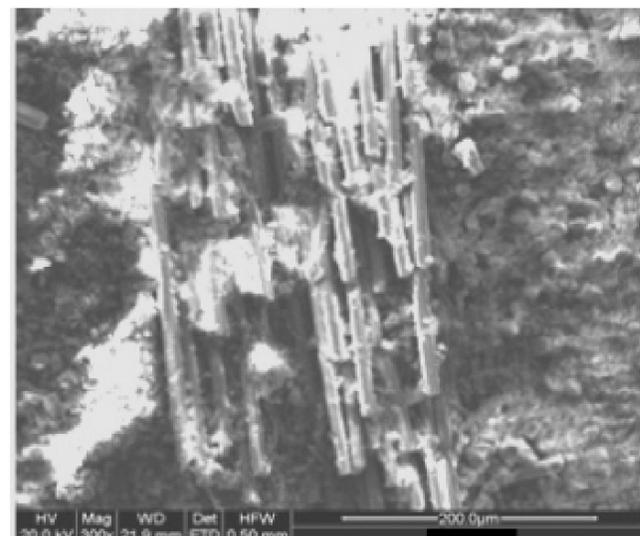
**Figure 6(c) : SEM of (GV<sub>3</sub>) at load 30N & speed 2m/s**
