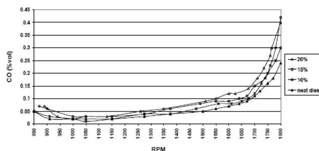
Figure 4 : CO emission of neat diesel and emulsified fuels with 10, 15 and 20% water content.
