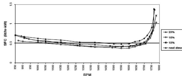
Figure 3 : Pure specific fuel consumption using emulsified fuels and neat diesel
