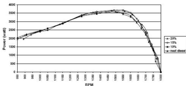
Figure 1 : Output power of neat diesel and emulsified fuels with 10%, 15% and 20% water content
